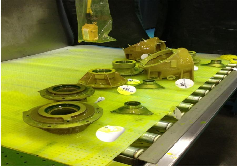
*When the time set is up they are rinsed off and then put in a dryer.*
