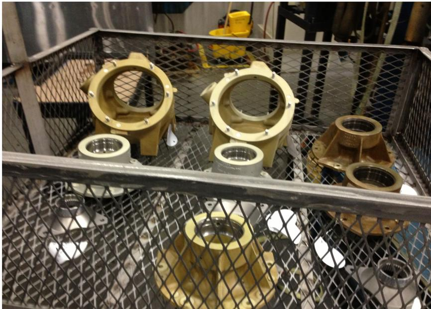
*After going through the wash cycle they are sent to dye penetrant.*
