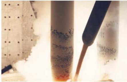
An electrode supplies power (center) while raw materials are added to a furnace via feed chute (right).
